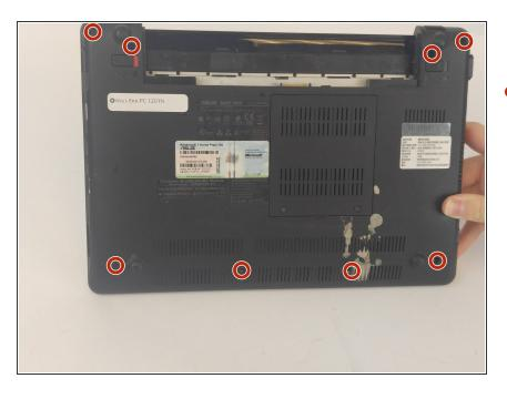
Turn the netbook over and remove the eight 6.5mm screws using the J0 Phillips head screwdriver.
