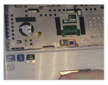
Flip up the retaining flap on the ZIF connector. Then, pull the blue tab for the touchpad connector before removing the cover plate completely.
