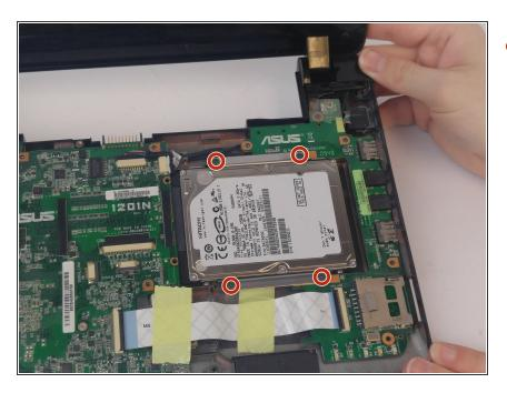
Remove the four 4.6mm screws with the J0 Phillips head screwdriver.
