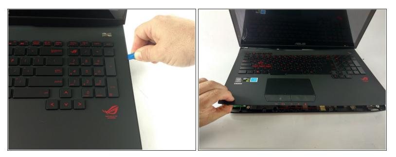
• Use the plastic opening tool to pry the keyboard from the base of the laptop.
