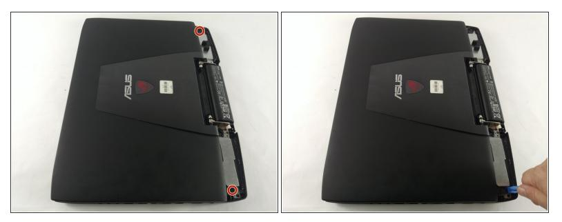
Remove the two 6.8 mm screws underneath to back panel, highlighted in the photo, with a Phillips screwdriver.
