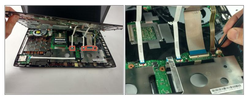
A Lift the keyboard carefully, otherwise the ribbon connectors may tear or break
