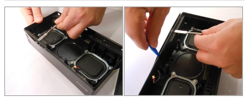
Using both the plastic opening tool and metal spudger gently pry open the cover from the top of the speaker.
