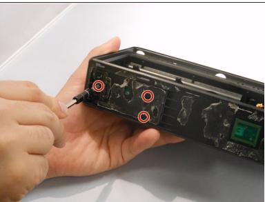
Using the Phillips #00, unscrew the three 3.32mm screws keeping the button board in place.
