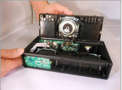
Using the plastic opening tool, flip open the speaker panel.
