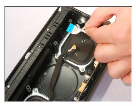
Gently tug on the plastic ribbon connected to the bottom side of the speaker to unplug it.
