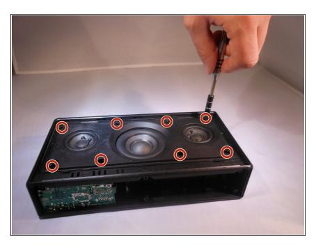
Remove the eight 0.5mm Phillips #1 screws from the speaker panel.
