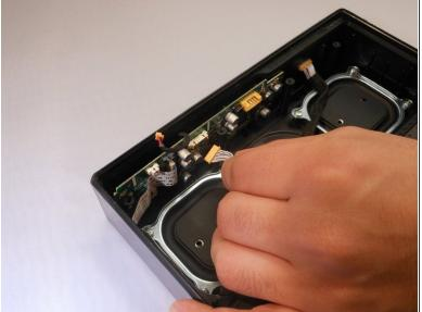
• Unplug the cord connected to the motherboard by squeezing the plastic sides.
