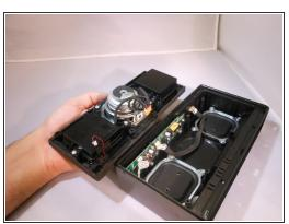
Unplug the 6-pin speaker connector and 2-pin microphone connector from the motherboard by squeezing the sides of the plastic ends.
