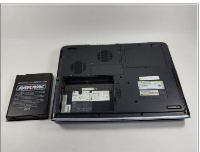
Using two fingers, pry the rest of the battery out of the socket.
