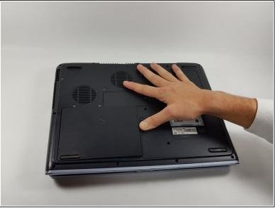
Press and slide up the battery release tab with your thumb until the battery pops out of place.
