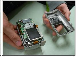
Use the blue opening tool to loosen and separate the back cover from the camera.
