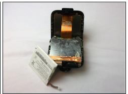
⚠ This step shows the use of an incorrect tool. Only use ESD safe tools when handling the battery.
