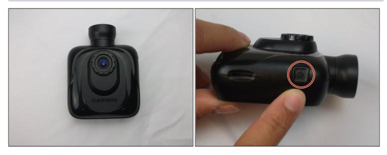
$\triangle$  Be sure to turn off the Dash Cam by pressing the power button.
