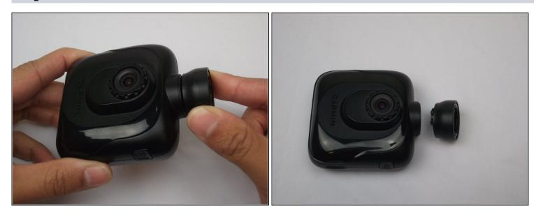
• Remove the Dash Cam socket piece.
