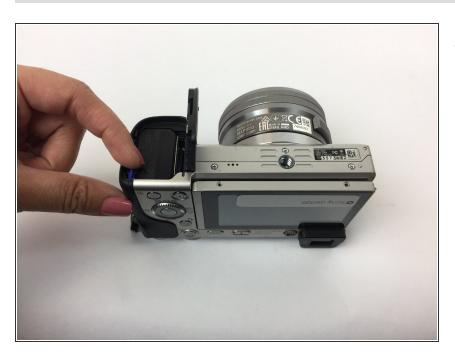
Push the latch back to release battery.
