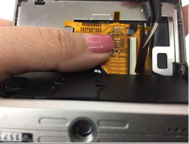
Remove the larger ribbon cable. This may require extra force that could damage the ribbon cable.
