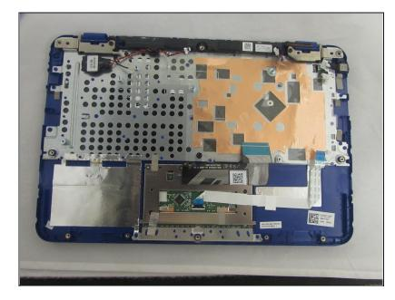
• Remove the motherboard by gently lifting upwards from the edges.
