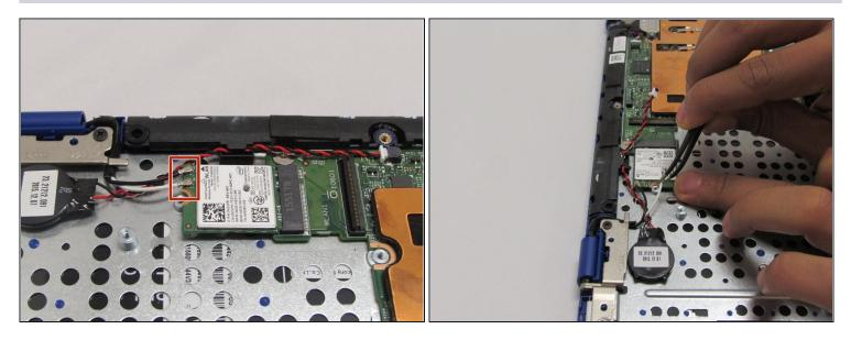
• Using the <u>tweezers</u>, pull the white and black wires off of the WiFi Chip.
