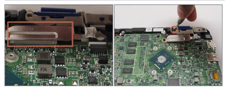
• Use the phillips screwdriver with the PH00 head to unscrew the one 3mm screw. Then, remove the bracket.
