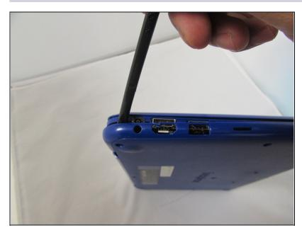
• Use a spudger to pry around the base edges of the back cover to loosen it from the laptop.
