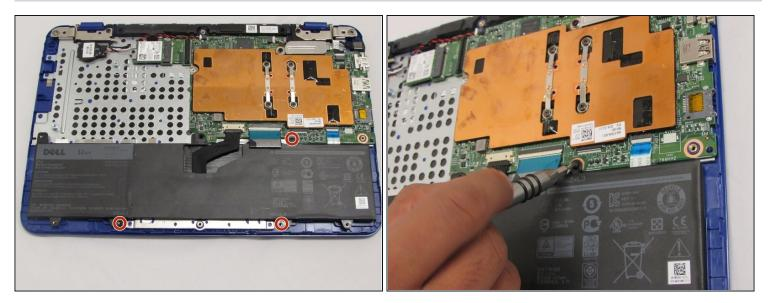
• Use a Phillips screwdriver to unscrew the three 4 mm screws securing the battery.
