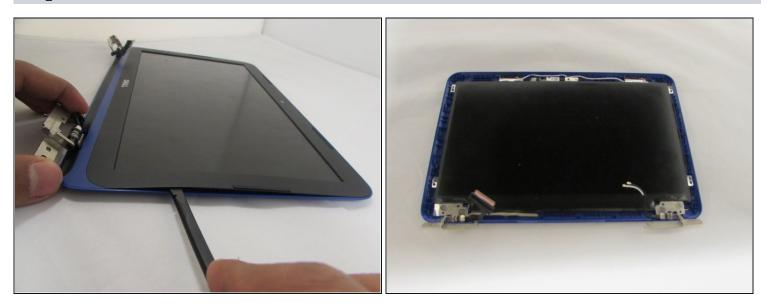
• Carefully remove the LCD Bezel with your regular black nylon spudger tool by bringing it all the way around the outer edges of your screen.
