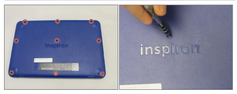
• Use a Phillips screwdriver to unscrew the nine 6.8 mm screws securing the back cover.
