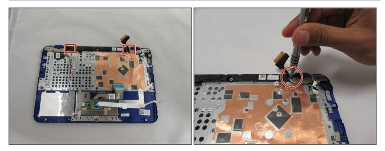
• Remove the two screws that hold down the LCD hinges.
