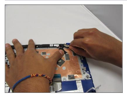
• Pull the hinges back and remove the screen.
