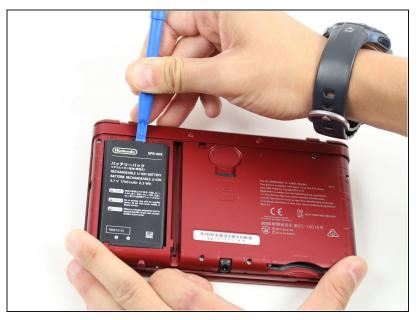
• The battery is located on the left hand side of the 3DS - to remove, use the small gap located at the top-middle and pull up with a non metal pointed tool.
