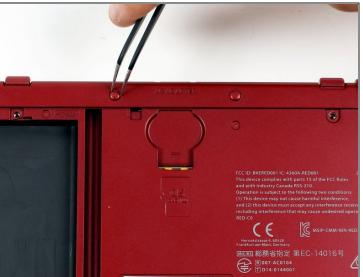
Using tweezers, carefully pop out the rubber bumpers located at the top side of the 3DS.
