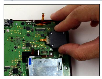
Lift the circle pad casing upward to remove it. There will be some friction, but it should not require excessive force.
