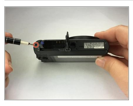
Remove 1 black Phillps 4 mm screw using a Ph000 screwdriver tip from under battery cover.
