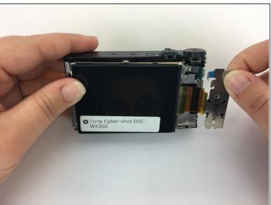
Pull blue band holding the control wheel away from the camera body.
