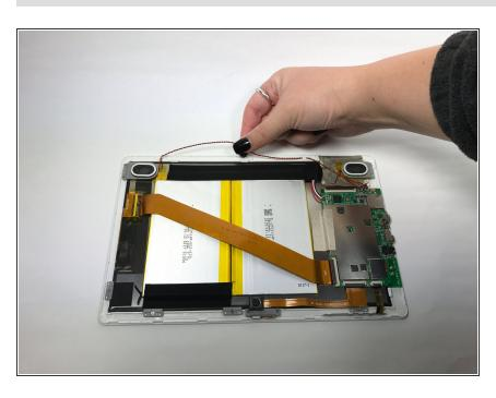
Unhook the woven red and black wires from the plastic hooks that hold them in place against the front panel
