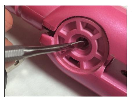
• Use the metal spudger to push the center pin through to the other side.
