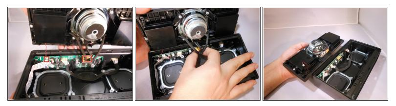
Unplug the 6-pin speaker connector and 2-pin microphone connector from the motherboard by squeezing the sides of the plastic ends.
