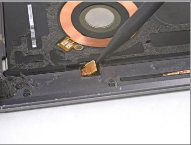
• Use the point of a spudger to pry up and disconnect the wireless charging coil connector.
