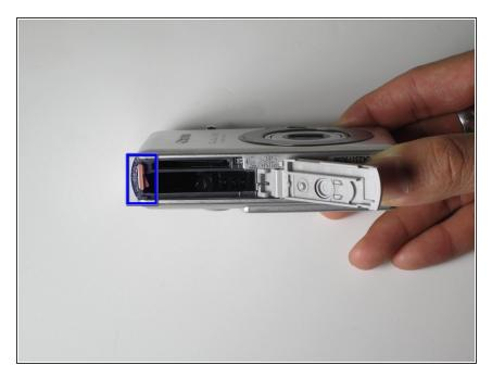
Push in the orange clip (indicated by the blue box) to eject the battery.
