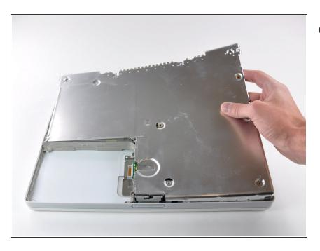
Lift the bottom shield off.
