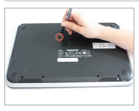
Use a J0 bit tipped screwdriver to unscrew the one 6 mm Phillips screw on the RAM cover.
