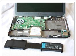
• Lift the tiny black tab and pull the battery out at a slight angle.
