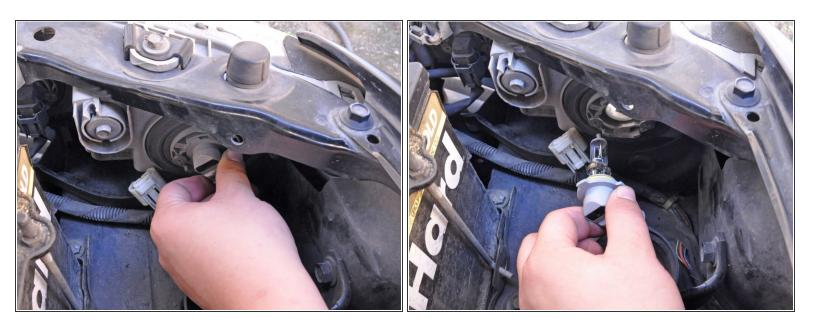
Turn the head light bulb counterclockwise and pull it straight back to remove it.
