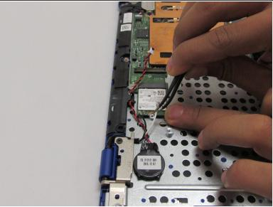
Using the tweezers, pull the white and black wires off of the WiFi Chip.
