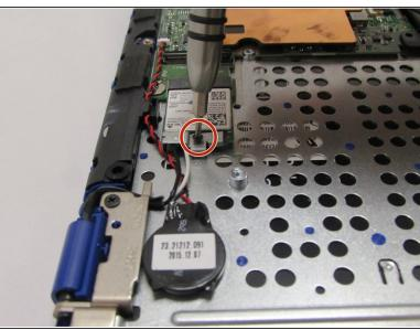
Use the phillips screwdriver with the PH000 head to unscrew the 3.8mm screw.
