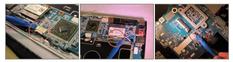
• Locate the wires and connectors and remove them from the motherboard.
