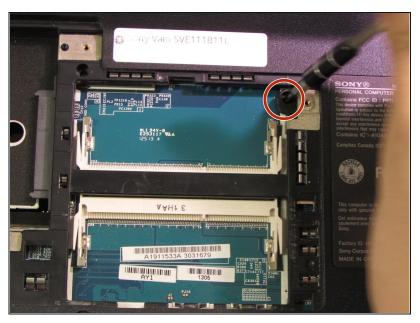
Remove the 6.7 mm screw that holds the keyboard assembly in place.
