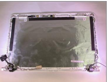
• Gently lift the screen assembly up and out.
