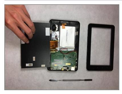
• Carefully lift the screen and set it face down on a soft surface to not scratch it.
