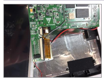
Remove the 2 ribbons from the motherboard by pulling the black connections out of the white connections on the motherboard.
