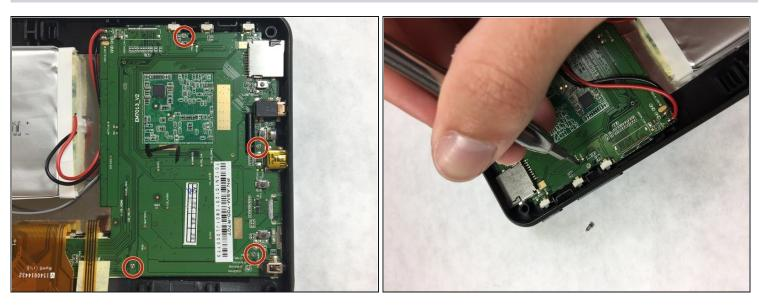
• Remove the 4 3.8mm phillips #000 screws holding on the motherboard using the PH000 phillips head.
