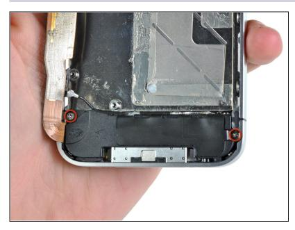
Remove the two 2.4 mm Phillips screws from the sides of the speaker enclosure assembly.
