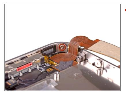
• Remove the 1.5 mm Phillips screw near the dock connector cable.
