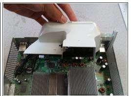
To remove the fan covering, use a flat head screw driver as shown to gently pry it off
