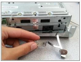
To pop off this button, use the flat end of a spudger or flat-head screwdriver.
