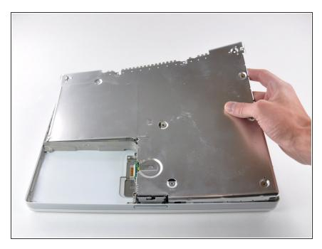
• Lift the bottom shield off.
