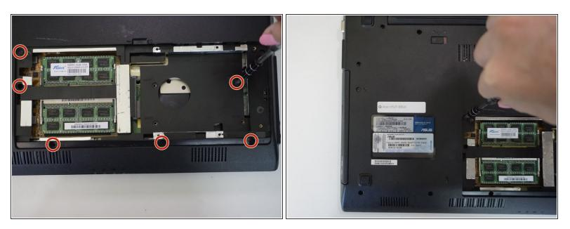
• Unscrew six 3mm Phillips screws in the RAM and hard drive compartment with the J1 screwdriver.
