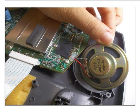
Solder your replacement speaker into the circuit. For assistance with soldering refer to <u>iFixit Solder and</u> <u>Desolder Guide</u>.
