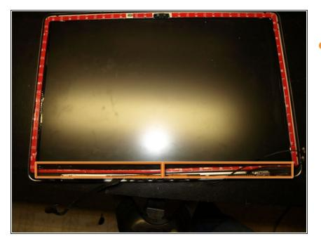
Apply the two 3mm x 170mm strips on the flange, red side up, between the bumper and screen at the bottom of the display assembly.
