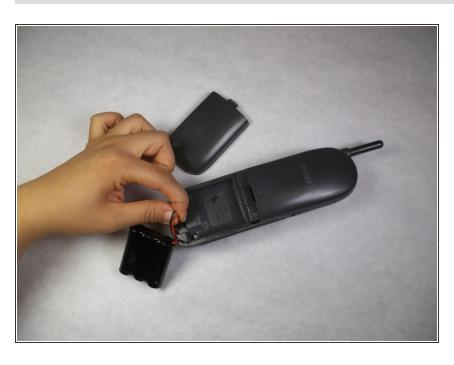
Remove the rechargeable battery pack (BP-T18) by pressing down on the power cable connector and pulling at the same time.
