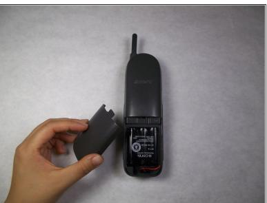
Remove the battery cover by placing your thumb on the cover and gently push towards the base of the phone.
