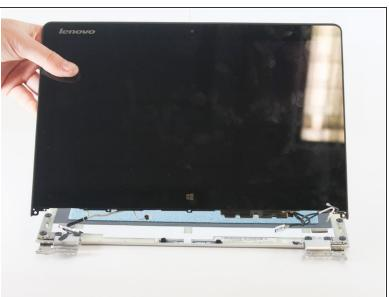
Remove the LCD by carefully pulling away from the hinges and upwards.
