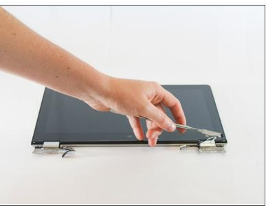
Remove the LCD hinge cover by gently prying the pieces with a plastic spudger and lifting the hinge cover up and out.
