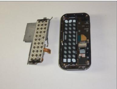
• The keyboard chip is located on top of the device. Pry the keyboard off of the case with the plastic opening tool.
