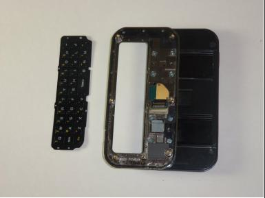
To remove the keypad, slide out the display, and poke the keypad out.
