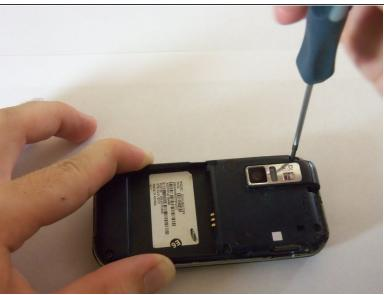
Use a Phillips #00 screwdriver to remove the six 4mm screws.
