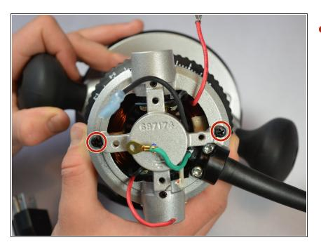
Use a phillips screwdriver to unscrew the two black 50 mm screws.
