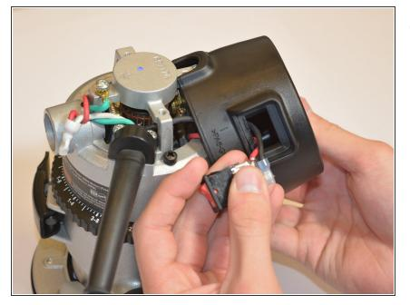
Push the power switch through the top of the router. The power switch should now be completely detached from the router (besides the wire connections).
