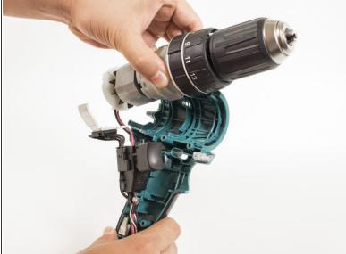
Gently grip the front of the motor assembly and pull it out of the plastic casing.
