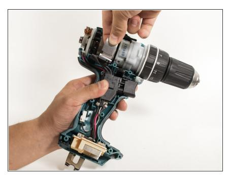
Pull the silver metal clip located towards the back of drill away from the motor assembly.
