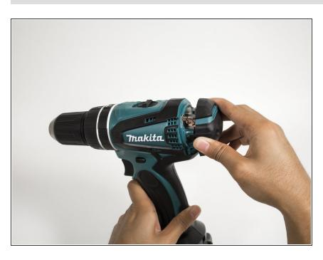
Apply slight pressure to the sides of the backplate and pull away from the drill.
