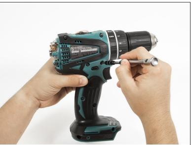
Unscrew the nine 18 mm screws from the outer casing using a Phillips PH2 screwdriver.
