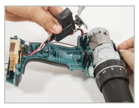
Pull the black trigger assembly away from the drill.
