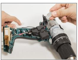
Pull the silver metal clip on the motor away from the drill.
