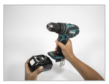
Slide the battery forward while pressing down on the white batteryrelease button.
