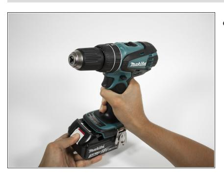
Press and hold the white release button located on the front of the battery.
