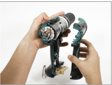
Apply slight pressure to the sides of the outer casing and pull away from the drill.
