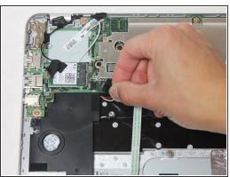
Pull the red and white wires out of the socket above the left speaker to disconnect the speakers from the motherboard.
