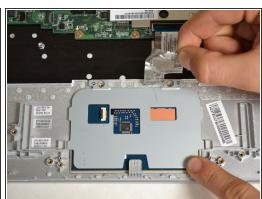
Peel back the aluminum foil piece on the top right corner of the touchpad.
