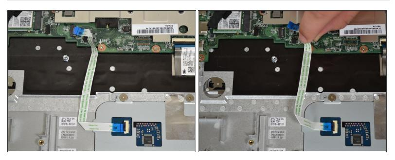
Detach the ribbon cable connected to the motherboard by gently pulling near the top fold.
