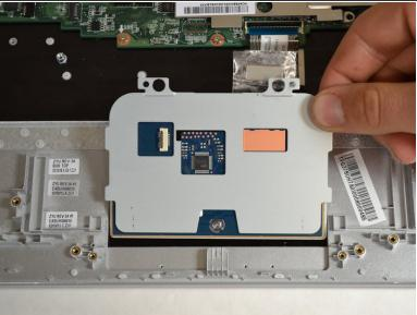
Push down on the bottom right corner and slowly lift up in the upper right hand corner until the touch pad comes out.
