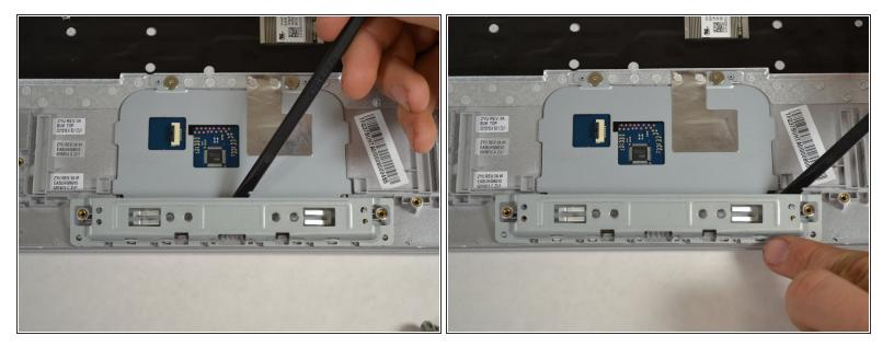
• Use the spudger to push up on the metal cover below the touch pad until it reaches 90 degrees then pull up to detach.
