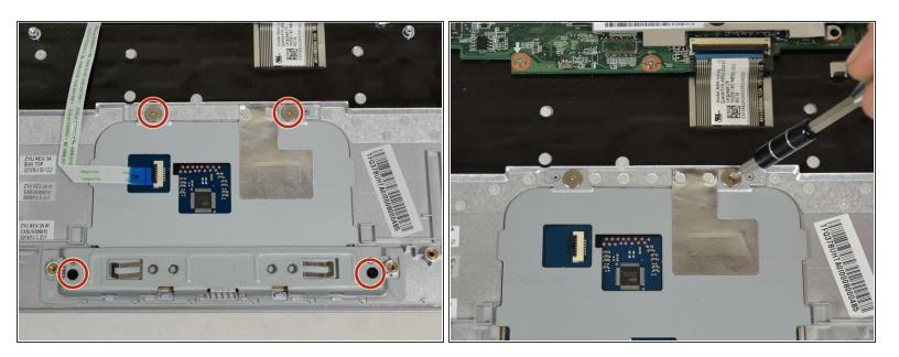
• Remove all four 3.70mm screws around the edges of the touchpad using a Phillips #0 screwdriver.
