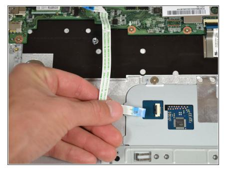
Detach the ribbon cable connected to the touch pad by gently pulling near the bottom fold.
