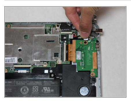
Pull the charging port out by pulling up on the cable that connects the port to the motherboard.
