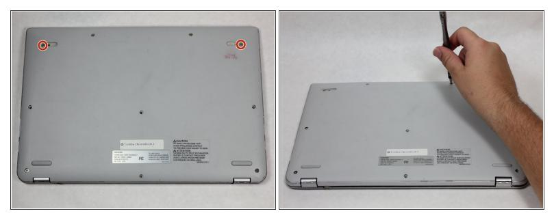
Remove 2 hidden Phillips 8.25 mm screws located underneath the rubber grips at the back (opposite the hinges) with the Phillips #0 screwdriver.
