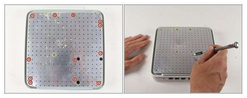
• Remove the ten 3mm screws with a Phillips #00 screwdriver.
