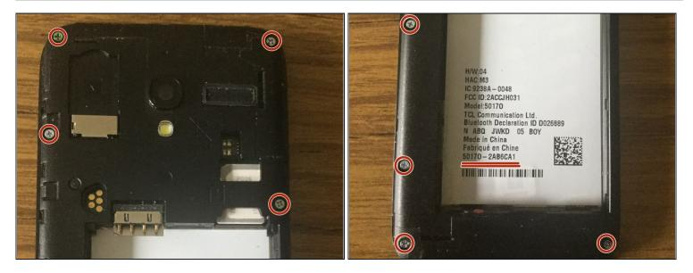
• Once you have the back removed and the battery set aside, you have 4 (long screws) at the corners, and 4 (smaller) screws in the middle. Set these aside in a safe place. (I used the back of the phone itself)
