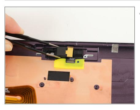
Use tweezers to gently lift the right camera, which is the rear camera, out of the device and set it aside.
