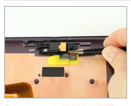
Using tweezers, gently pull the left camera, which is the front facing camera, and small attached ribbon cable off the device and set them aside.
