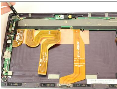
Using a Phillips #00 screwdriver, remove the six 2.5mm screws and set them aside.
