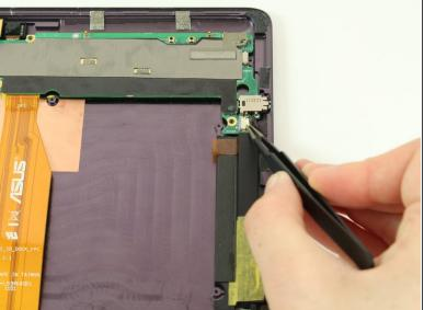
Using tweezers, pull the black part of the connection between the mother board and speakers out of the white part of the connection.
