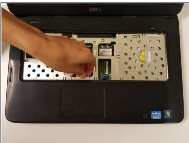
Lift the entire surface (palmrest casing) to expose the motherboard underneath.
