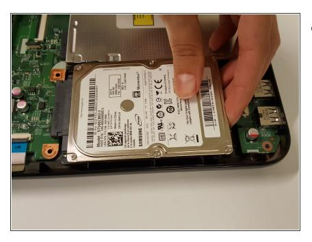
Slide the hard drive right and up to remove it from the laptop.
