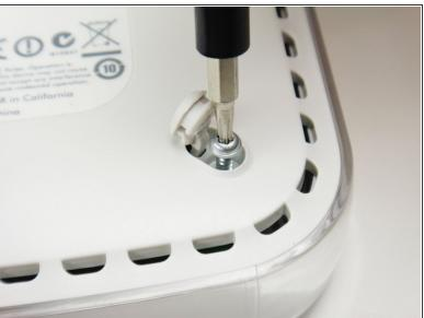
Unscrew the four 11.8 mm T-8 torx screws from the bottom of the router.
