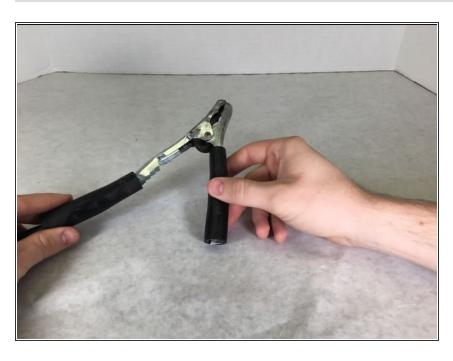
Slide the rubber grip back onto the handle.
