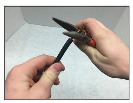
Clip the excess frayed copper strands from the cable using the wire cutters.
