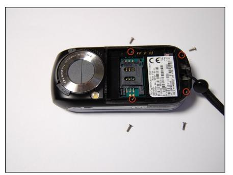
Remove the four 6 mm screws from beneath the battery using a Phillips #00 screwdriver.
