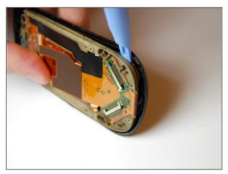
Pry the screen assembly from the main case using the iFixit opening tool.
