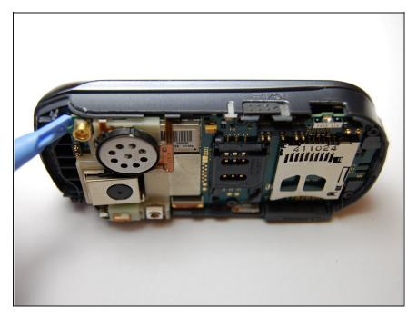
Use the iFixit opening tool to loosen the motherboard from the phone.
