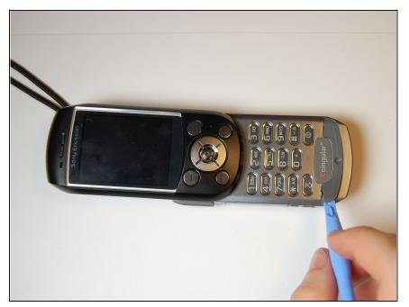
Remove the microphone cover using the iFixit opening tool.
