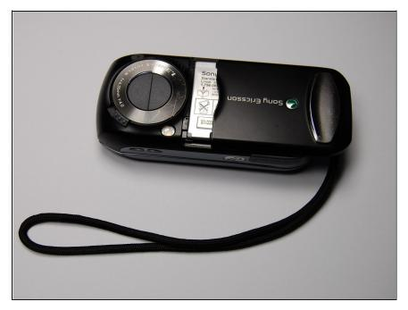
Remove the back cover by sliding it off.
