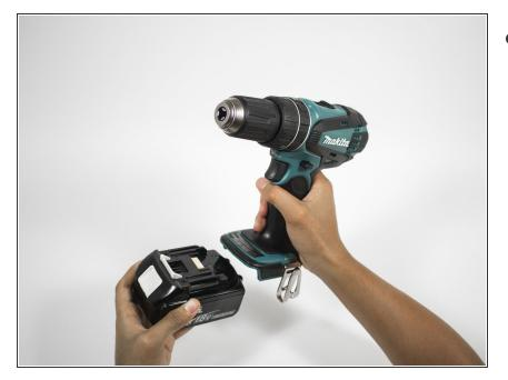
Slide the battery forward while pressing down on the white batteryrelease button.
