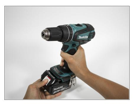
Press and hold the white release button located on the front of the battery.
