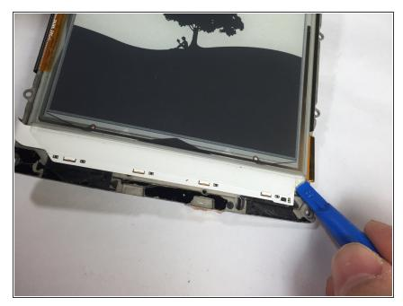
• The screen itself is glued to the midframe. If your replacement screen does not include the mid-frame, heat the screen with an iOpener and gently pry it from the mid-frame with a blue plastic opening tool.
