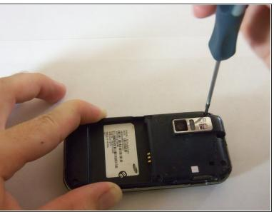
Using a Phillips#00 screw driver, remove the six 4mm screws holding the back case together.
