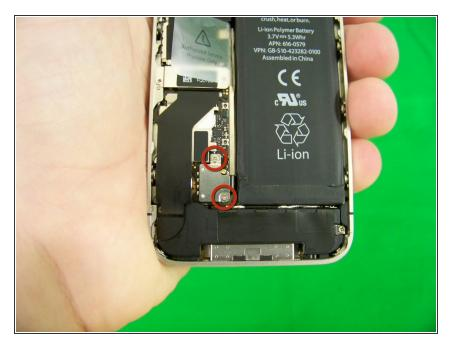
Using a #000 Phillips screwdriver, unscrew the 2 very small Phillips screws.
