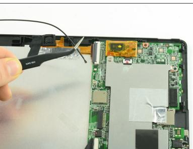
Use ESD safe tweezers to disconnect the antenna from the motherboard.
