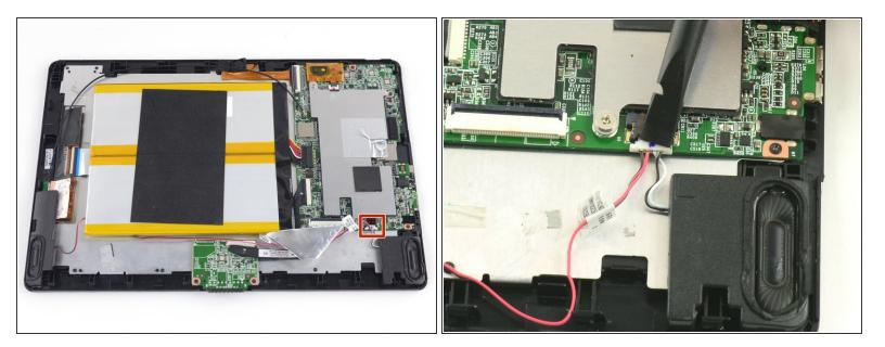
Use a spudger to release the speaker wires by pushing the bundled cabled connector away from the motherboard.
